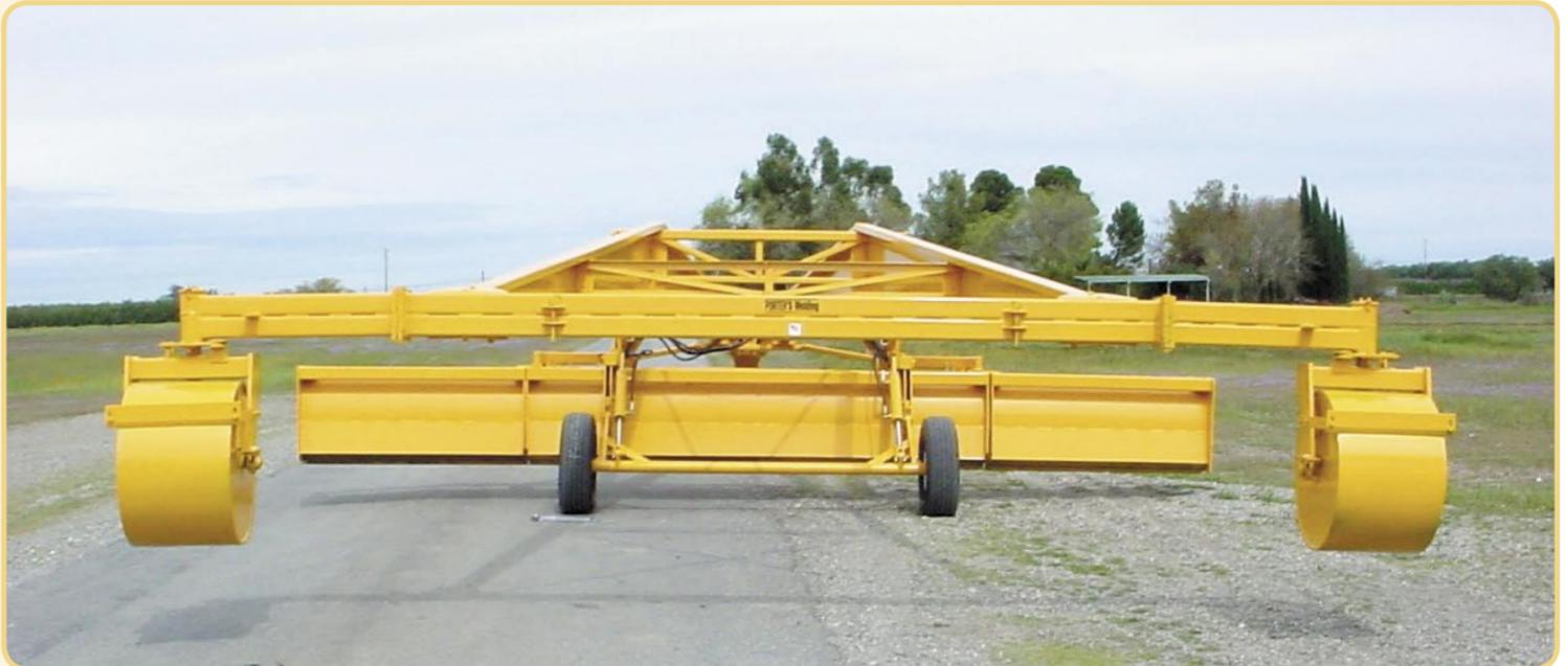
Porter's Tri Planes are fabricated out of high quality formed steel and completely welded for stability making this a Heavy-Duty frame.
