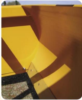
Rolled bucket creates less resistance for increased soil flow.
