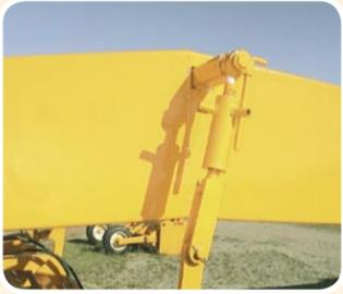
1/4" thick high grade steel for main frame.
