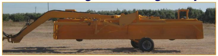
Save time with the new **Porter's Folding** Laser Drag Scraper. Same great features as the Laser Drag Scraper, but now with an easier and faster option than the transport wheels. This scraper is equipped with a hydraulic swing bucket and a modified tongue, so the scrapers does not have to be detached from the tractor. It takes approximately one minute to be converted from field to transport mode.
