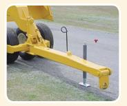
Reinforced hitch and heavy duty tongue for rugged pull.
