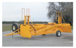
Fold down transport hitch from the side of the Laser Scraper. Hook transport hitch and hydraulic hoses to tractor. Safely move the Laser Scraper to the new location.
