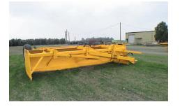
Fold the tongue and braces to the side of the Laser Scraper and lock with a pin.
