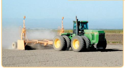
These scrapers are laser & GPS compatible with the option of single or dual laser receivers. When dual lasers are mounted on the Porter Laser Scraper, it allows each side of the scraper to act independently for enhanced accuracy.
