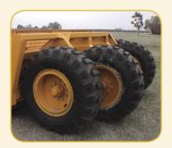
Four independently mounted, off-set tires allow the Carry-All to work at a high speed while remaining stable throughout the moving, loading and unloading of soil.
