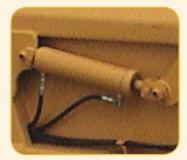
Heavy duty welded cylinders along with, high tensile braided steel wire, hydraulic hose protects against leakage and damage generating less possibility of down time.
